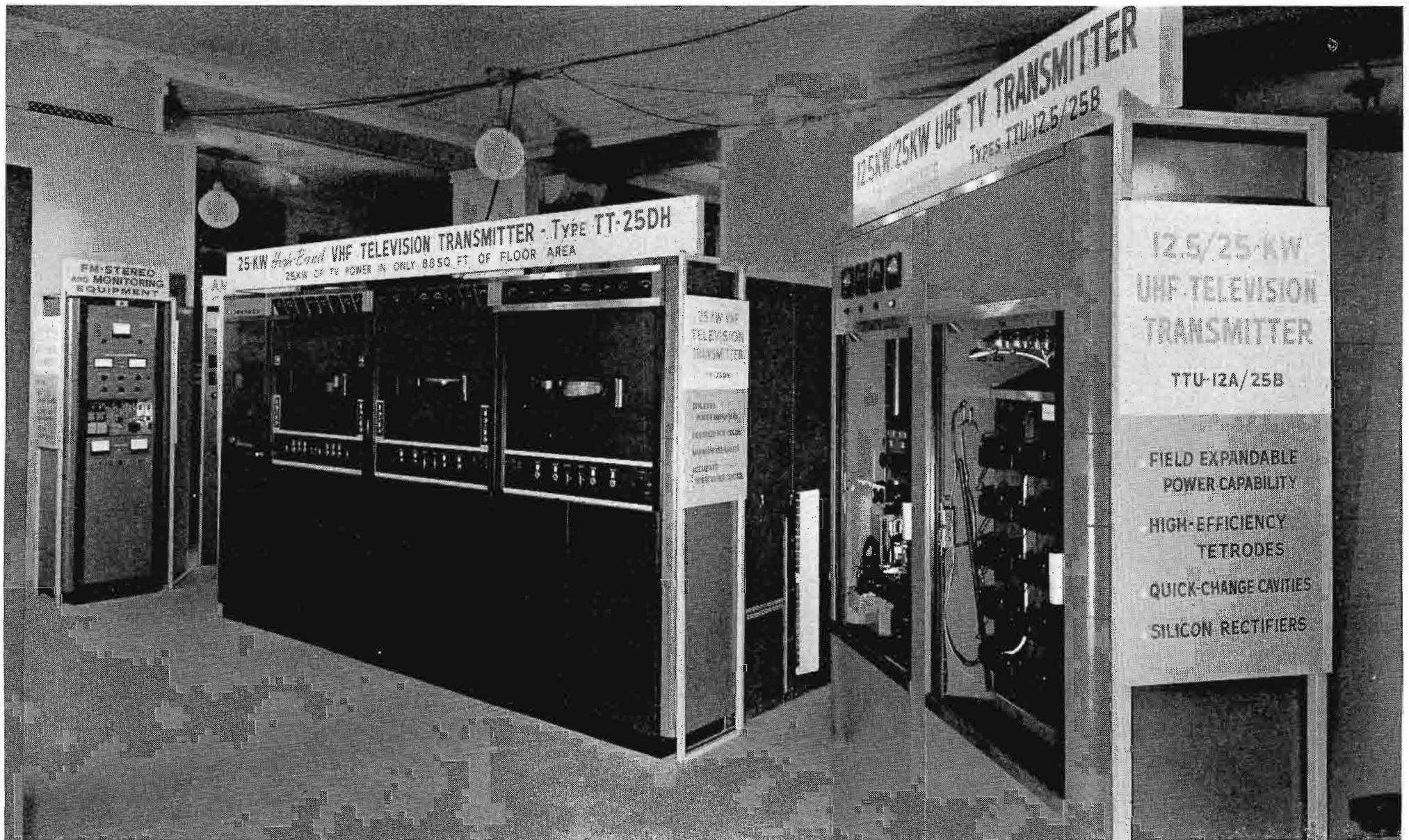
FIG. 7. Rack cabinet at left contains the BW-73A Multiplex Modulation Monitor; the TBM-3000 FM Frequency Monitor; the BTS-1A Stereo Subcarrier Generator and the BW-74 Modulation Monitor Stereo Adapter. The TT-25DH VHF Transmitter occupies center with the sections of the UHF TTU-12A/25B Transmitter at far right.
