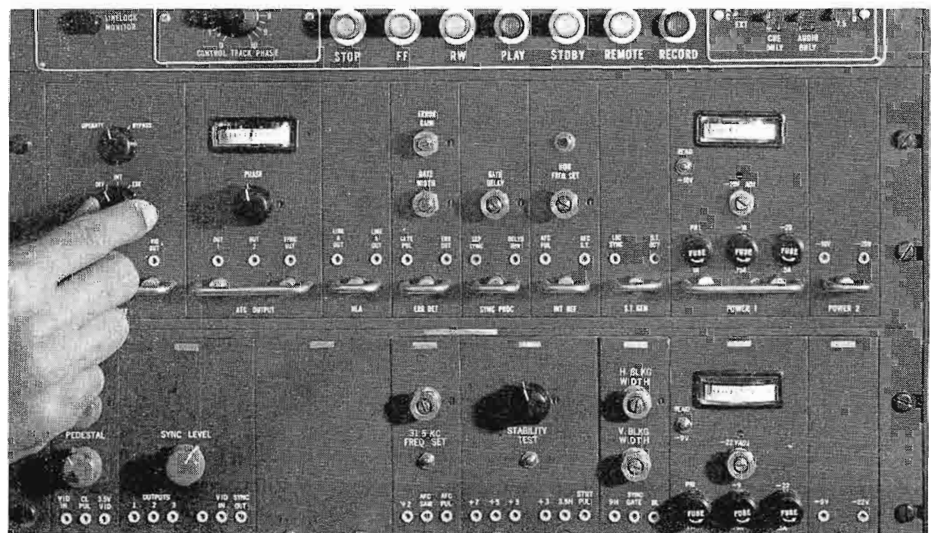
FIG. 9. The automatic timing corrector (ATC) is a fully transistorized unit of modular construction, similar to the processing amplifier and headwheel servo. Its purpose is to remove skewing and other geometric errors in the playback signal.
