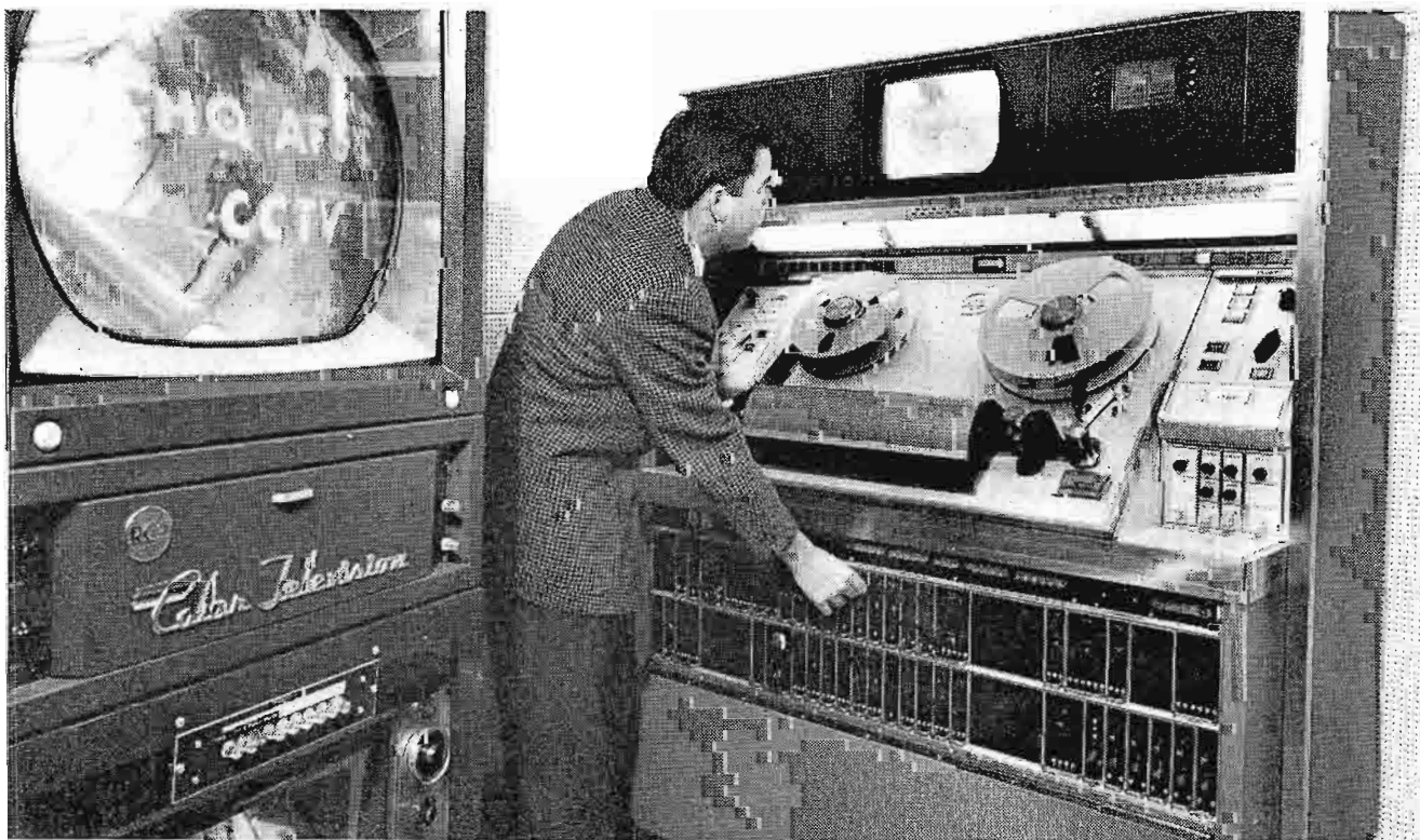
Andrews AFB video tape recording facilities include RCA TRT-1B and a transistorized TR-22 shown here.
