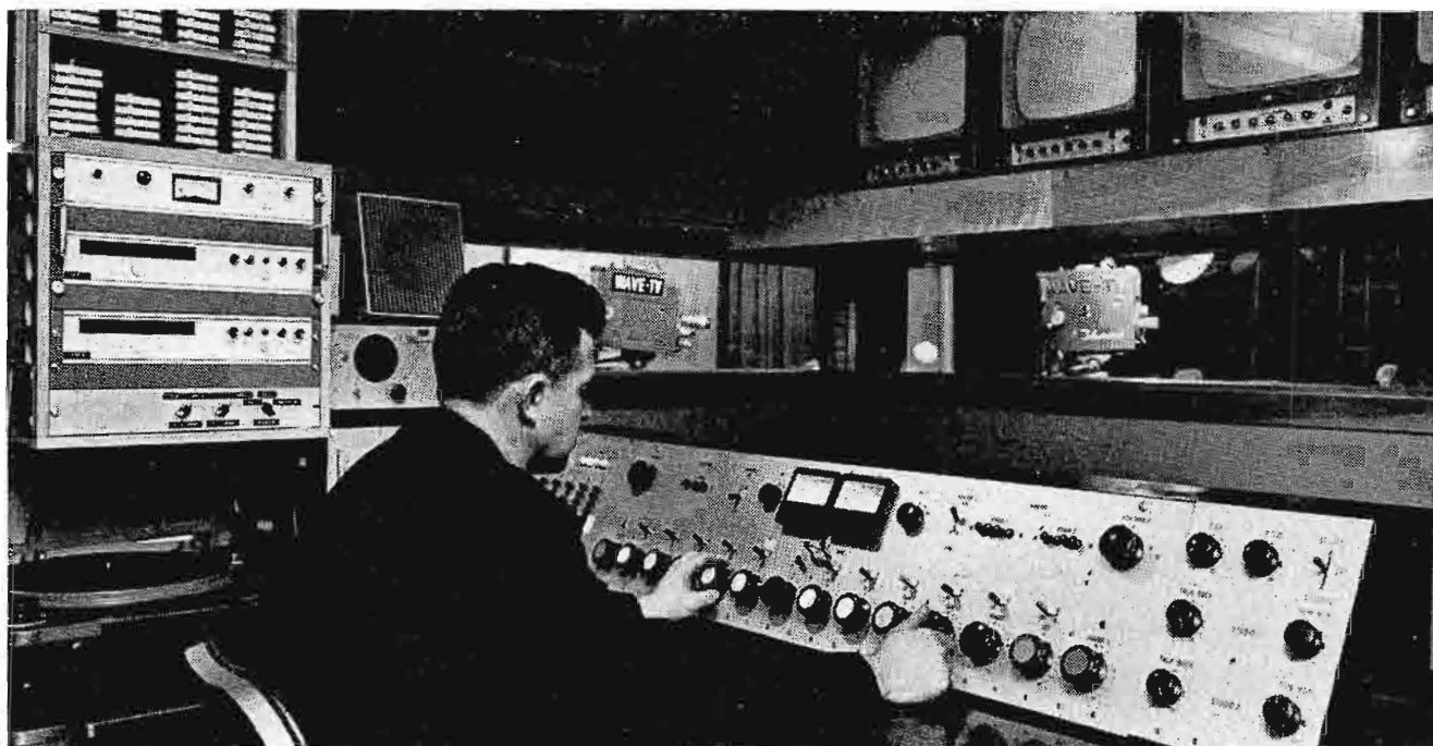
FIG. 21. Roy Parris at audio console in studio control room. It's duplicate of control in equipment room. Both were built by WAVE-TV. All amplifiers are housed in cubicle under console. At left is RT-7A Cartridge Tape unit.
