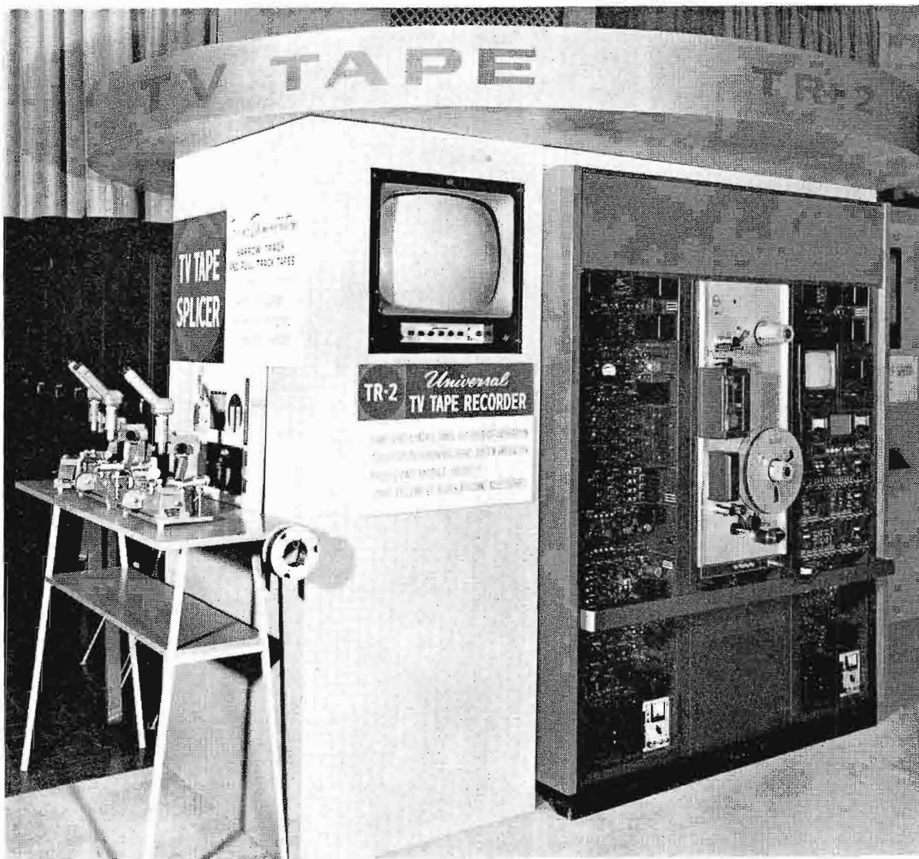
▲ FIG. 6. A basic quadruplex TV tape recorder filled out the tape equipment complement on display. The TR-2 shown here was fully equipped with Pixlock, two-speed operation, picture and waveform monitors, audio cue channel, and automatic timing corrector.
