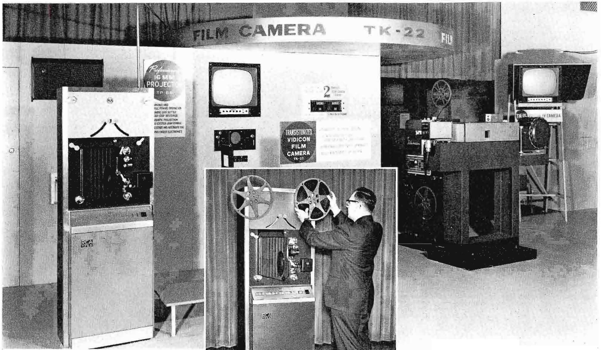
FIG. 11. This display demonstrated transistorized equipment for the modern TV film room. Included were a new vidicon film camera chain, TK-22 (right), and a new 16-mm TV projector, TP-66 (left and inset photo).
