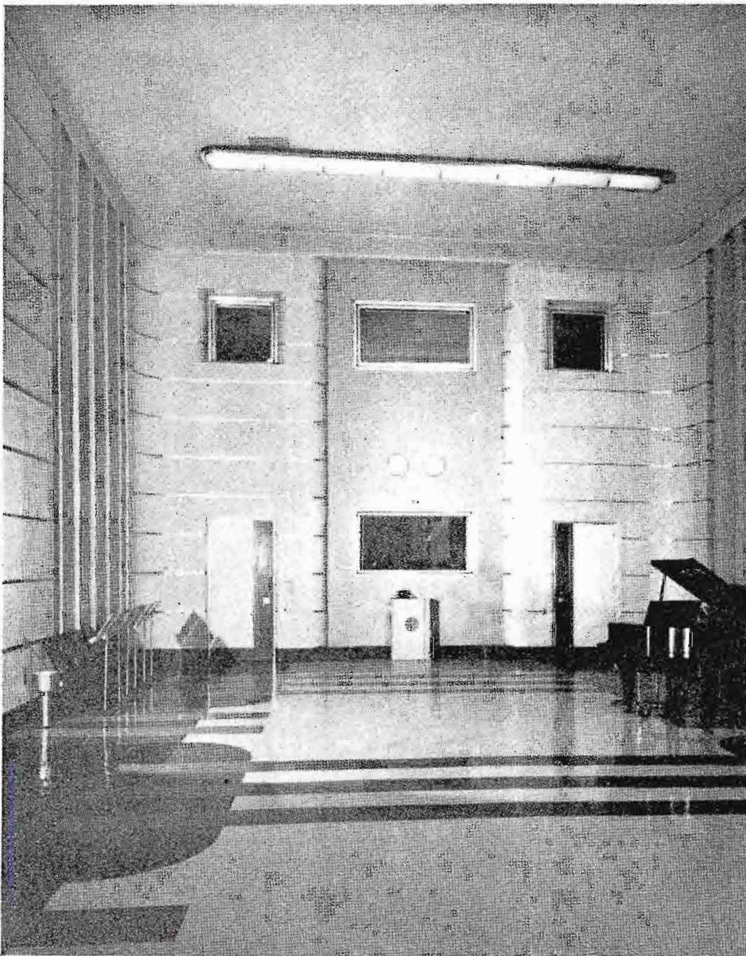
Studio A, 55 feet long, 32 feet wide, 23 feet high. Three windows at top are in observation gallery. Control room is in center below.
