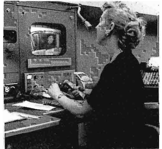
Close-up of teller position shows clear image of drive-in customer as it appears on 17-inch screen.
