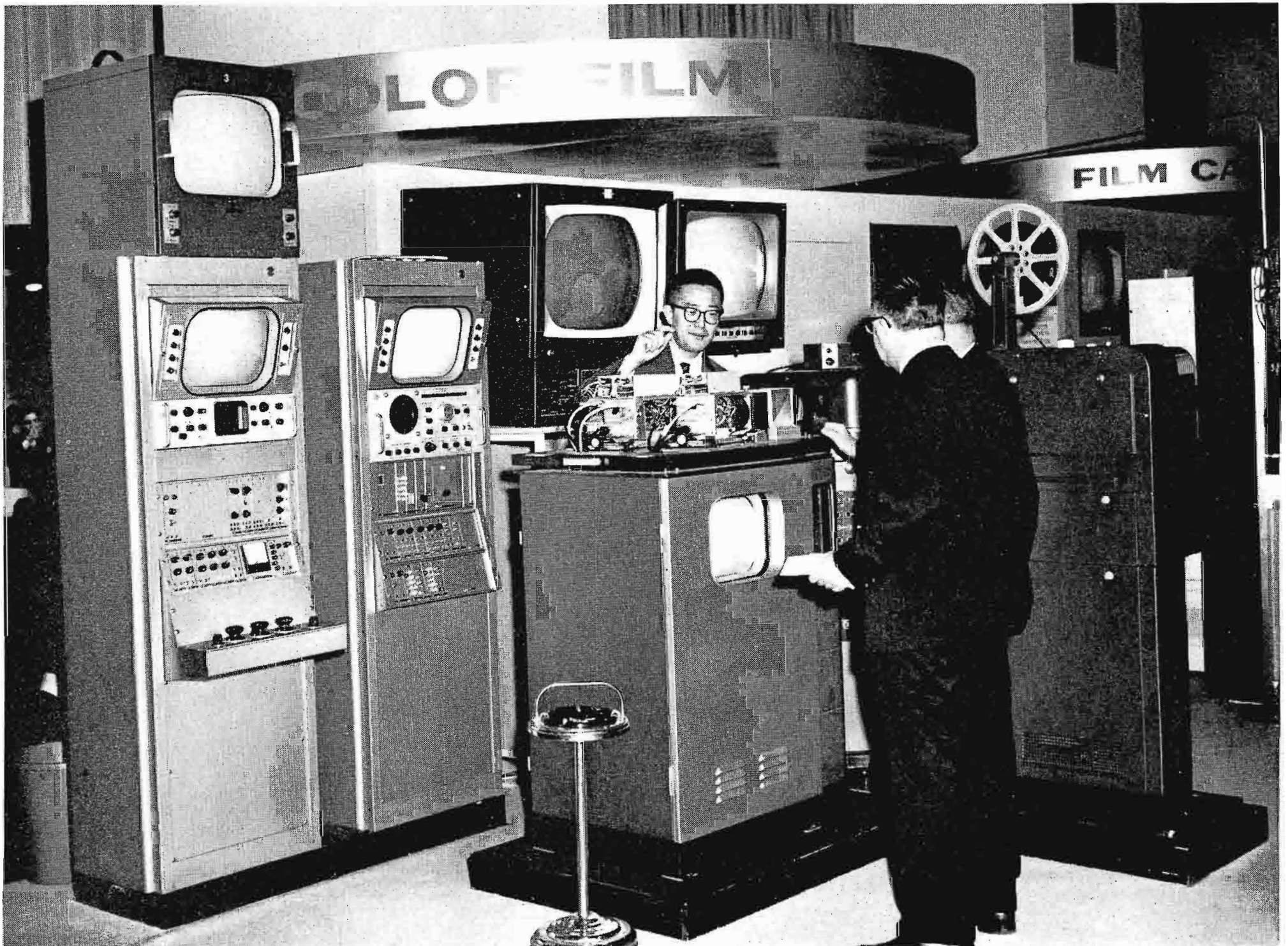
FIG. 10. A look at the improvements that lie ahead for color TV film, was provided by this demonstration of a 4-vidicon, transistorized color TV film system.
