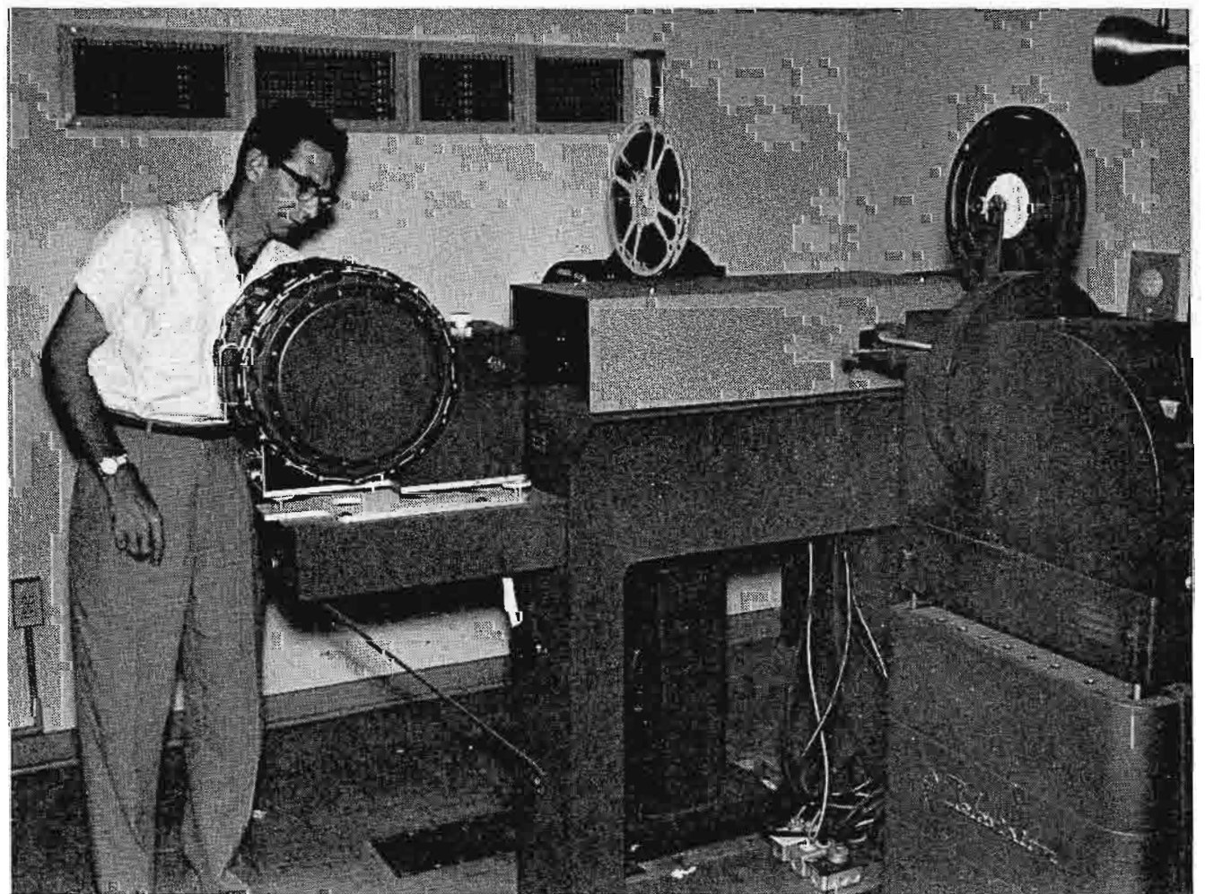
FIG. 8. WTVM film programming starts here. Herman Ragland loads the Type TP-7 Slide Projector which works into the TP-11 Film Multiplexer. The two 16-mm projectors are TP-16 units. The pickup is via RCA vidicon camera.
