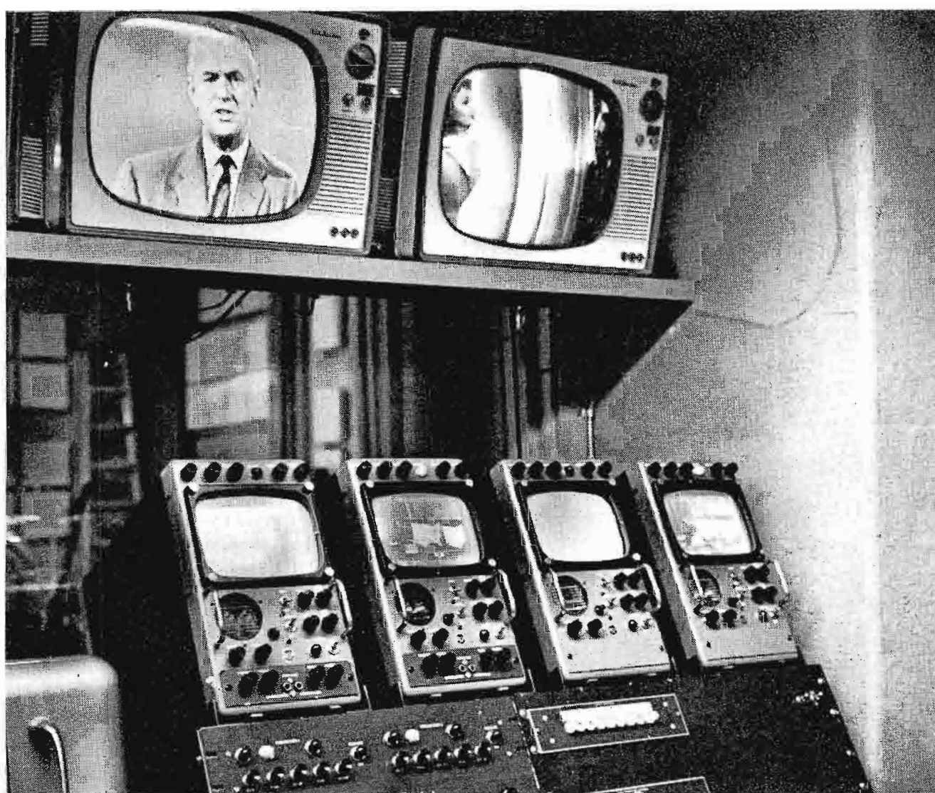
FIG. 7. Video control center, showing four TM-35 master monitors, controls for film system, and switcher-fader.
