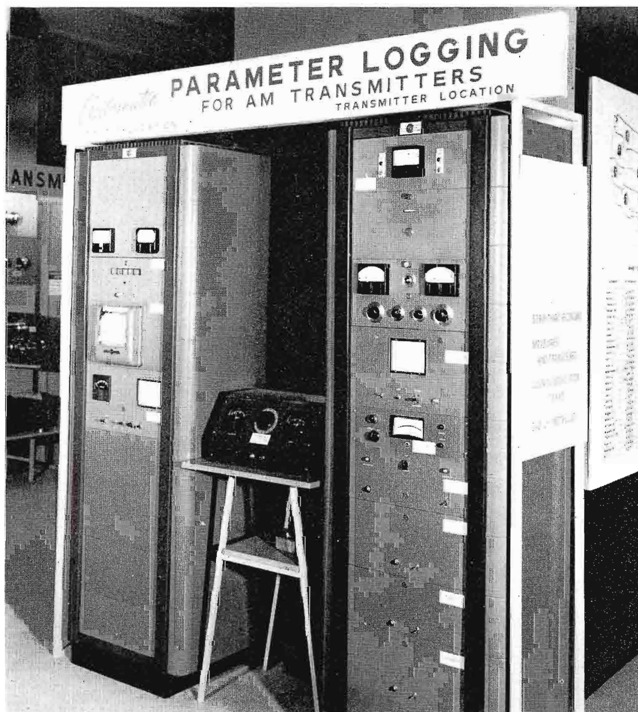
FIG. 8. Automatic parameter-logging equipment. Rack at left represents the studio portion of the system with the transmitter-located gear in the rack at right. The black box between the racks houses the demonstration controls for the automatic power-output control.
