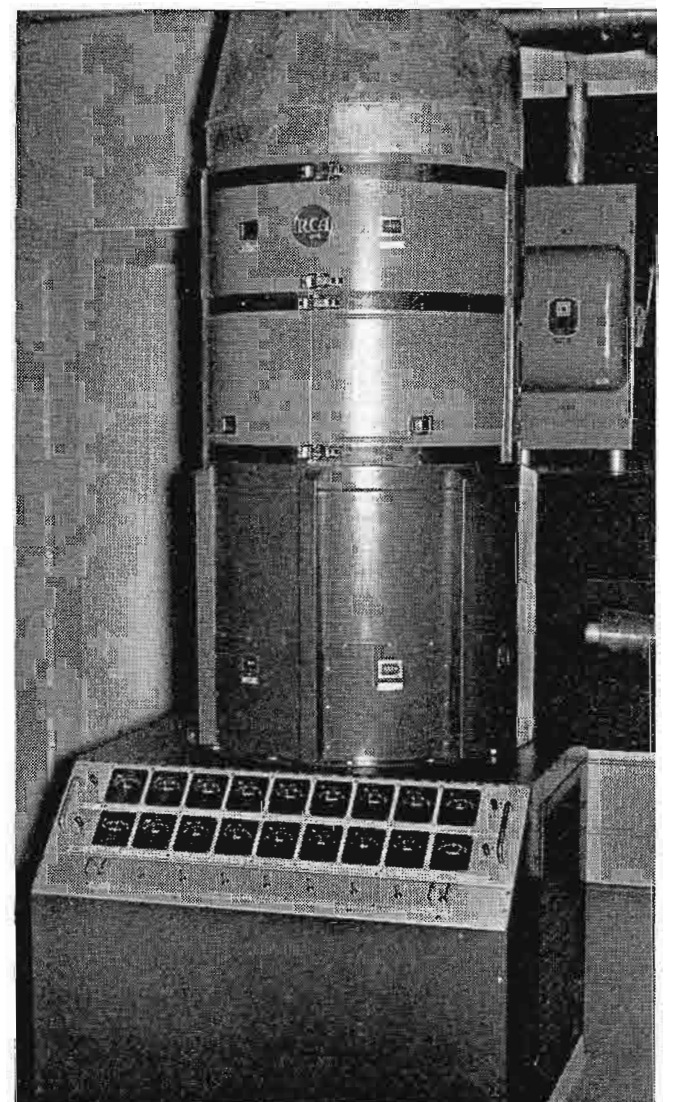
FIG. 13. One of the two r-f power amplifiers located to the rear of the driver of the transmitter (see FIG. 10). Primary-power switching devices on rear wall.
