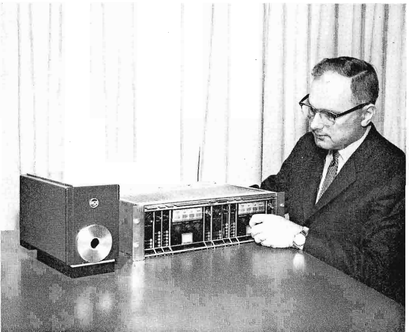
FIG. 12. Close-up of the TK-22 transistORIZED film camera and associated control and processing equipment. Control and processing units for two complete camera chains are mounted in the 5¼-inch rack frame shown.
