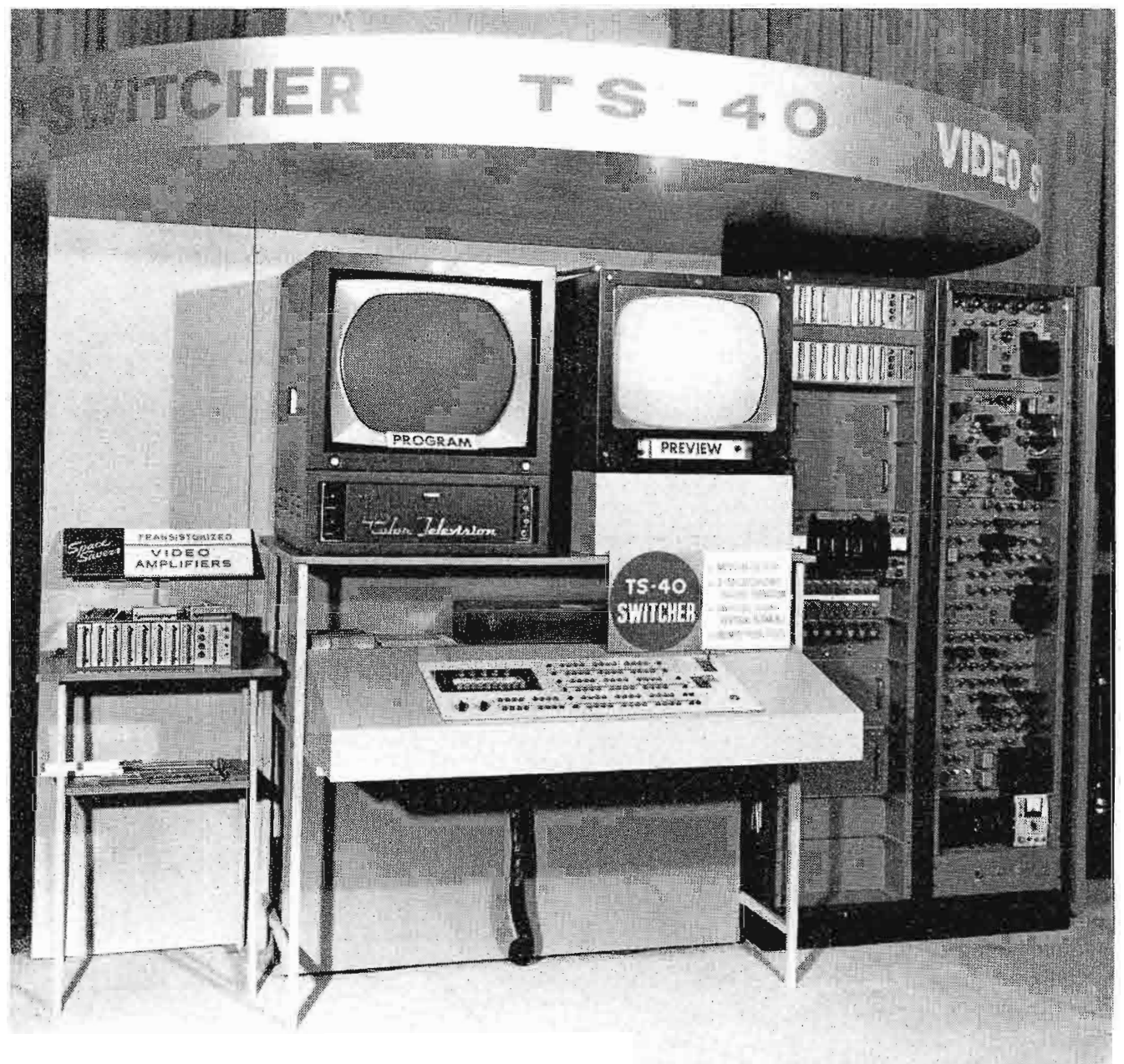
FIG. 13. Both color and monochrome performance of a typical TS-40 transistorized switching system with special effects was demonstrated in this display. A new line of transistorized Video Amplifiers (left) was shown for the first time.
